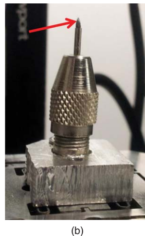
Fig. 1—(a) X-ray CT scanner imaging apparatus for shale core sample, (b) needle-mount sample setup for TXM studies. Red arrow points to FIB-prepared sample.
