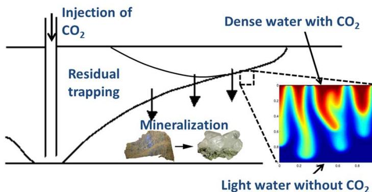
CO<sub>2</sub> plumes can migrate for long times after injection stops but are trapped by:
