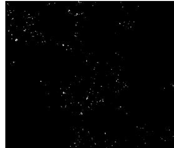
After image processing: bright particles, dark background and grain detections
