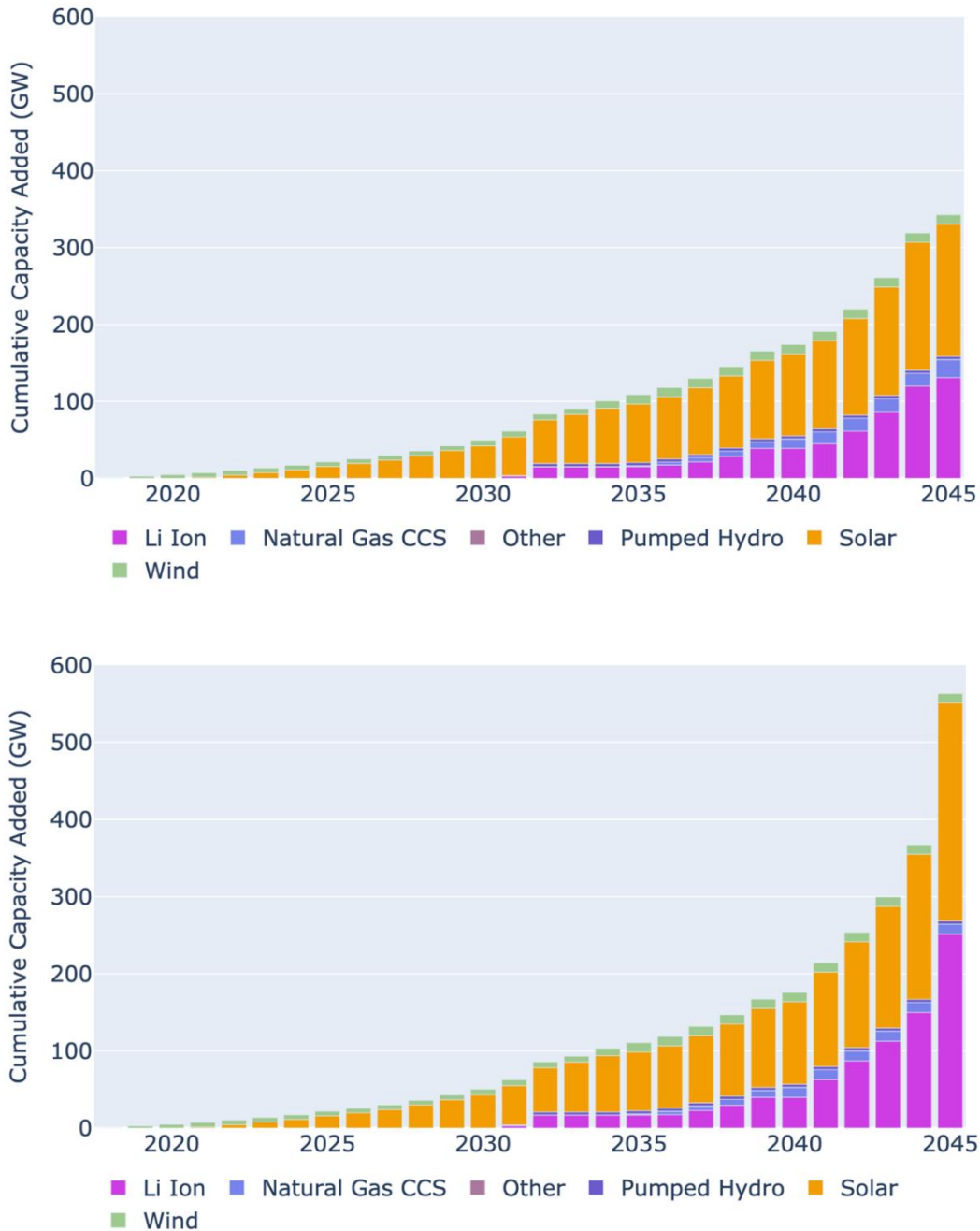
Figure 18: Electric capacity added with a CGC = 99% (top) versus a CGC = 100% (bottom), shown on cumulative basis. The 100% CGC does not allow for much NGCCS, resulting in a major buildout of solar and Li Ion storage.
