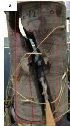
Instable CO 2 induced fracture (Bennour et al., 2015)
